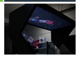
The monitor is placed in the upper part of the box The projection is heading downwards thanks to special industrial monitors enabling FACE DOWN placement For the perfect view on the 3D effect, the projection surface is situated at eye level
